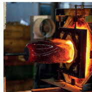
Production process of mouthblown glass
